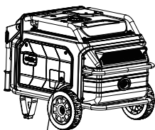
Oil service door
